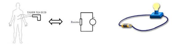
16. In any given electric circuit, the total power is limited by and cannot exceed the output of its power supply. A TASER X26 CEW's power source consists of a battery of two 3-volt cells (Duracell® CR123), such as those commonly used in some digital cameras.
