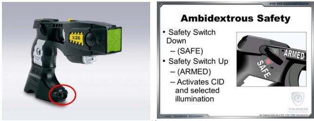
The TASER-Cam has a boot-up time of approximately 1.6 seconds after the safety is removed.
