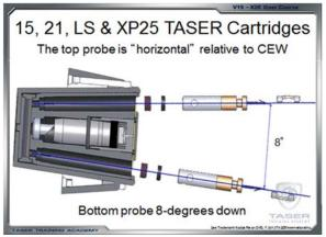
The optimum CEW deployment range is 7 to 15 feet. When deployed at close range, the probe spread may be insufficient to cause NMI.
